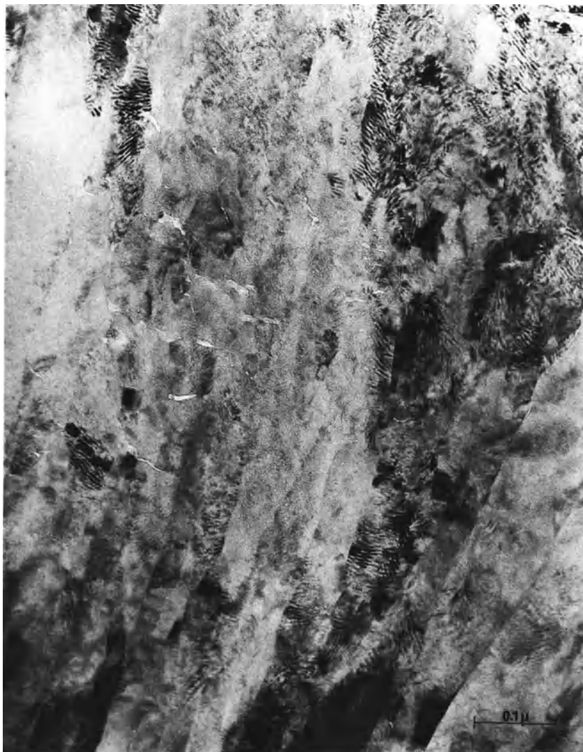
Fig. 87. Transmission electron micrographs of a section of a post-transition oxide film on Zircaloy-2 ion-thinned to obtain transparency. Note the elongated shape of the small crystallites, the presence of fine pores at crystallite boundaries, and the absence of gross cracks. 535
