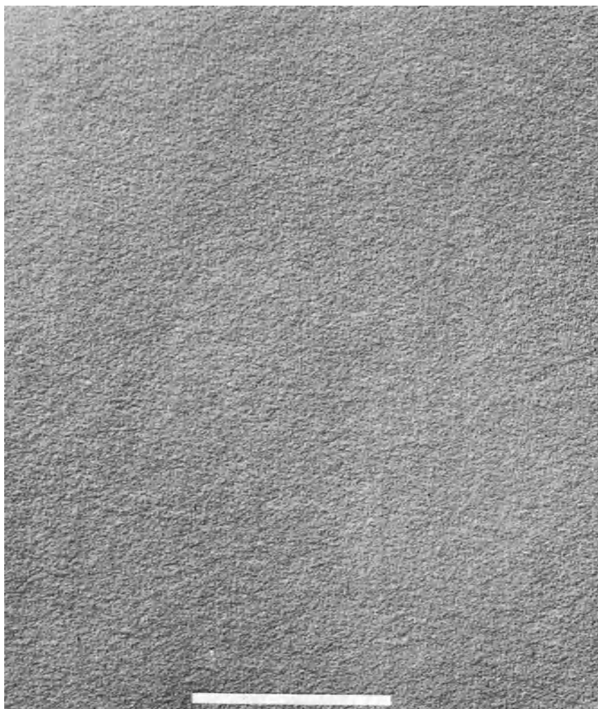
Fig. 8. Surface of fractured soda-lime glass.
